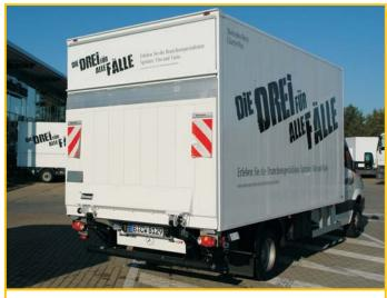
The best solution for your loading capacity: The standard tail lift X1A 750SL with 750 kg lifting capacity and only 168 kg own weight.
