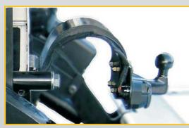
Option: Towing ball assembly, quick and easy installation, retrofittable.
