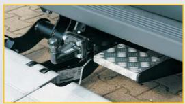
Options: step and towing ball coupling assembly, fast and straightforward assembly, can be retro fitted.
