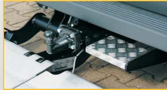
Options: step and towing ball coupling assembly, fast and straightforward assembly, can be retro fitted.
