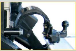
Towing ball coupling, quick and easy installation, retrofittable.
