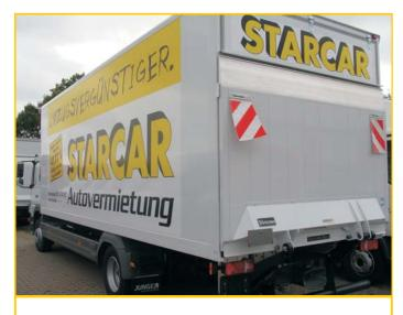
Particularly robust standard-tailgate X1A 1501 with 1500 kg lifting capacity for distribution vehicles.
