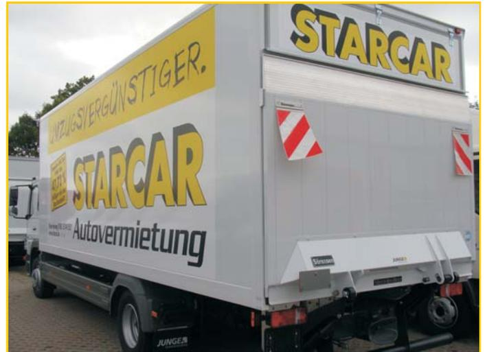
Particularly robust standard-tailgate X1A 1501 with 1500 kg lifting capacity for distribution vehicles.
