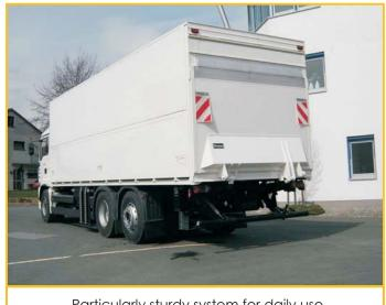
Particularly sturdy system for daily use in the food and beverage distribution, which can carry 2.500 kg at a load distance of 1.000 mm
