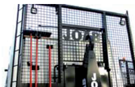
Impact tested front wall.
