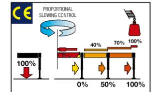
With a 3" TFT display and ergonomic keyboard, the crane operator can select optimum functional parameters. The system controls the stability with 2-step beam outreach monitoring and continuous slewing control.
