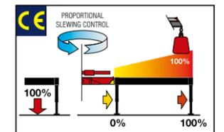
A 7" color display with integrated keyboard gives the operator a higher level of awareness of the crane operation and allows selection of the best parameters for effective use. The system detects the exact position of the beams and proportionally calculates the stability.
