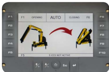
**Crane Automatic folding/unfolding.**
