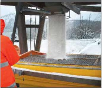
Every SOLID C spreader is equipped with a spinner for dry and wet spreading. Liquid spreading is possible by spraying liquid using the spinner or using a specially designed ramp with nozzles. Every parameter of spreading is controlled via the intuitive EPOS control unit located in the vehicle cabin.
