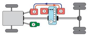
1 Gear box 2 Drive pump 3 Drive motors 4 Auxiliary pumps
